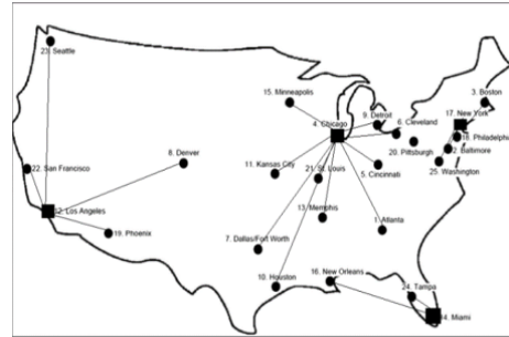
Figure 4: Hub location and allocating non-hub to hub nodes for sample 25d8 and \alpha = 0.2 (fixed cost was calculated based on relation (4.24))
